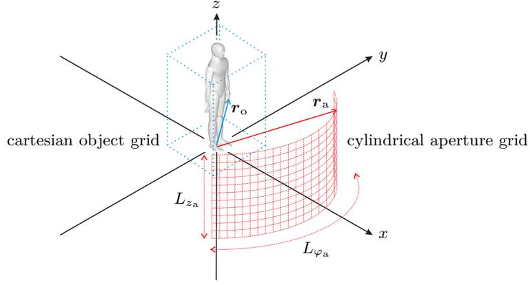
Fig. 1: geometrical setup: the cylindrical aperture grid is defined by the vector  $\mathbf{r}_a$ , the cartesian object grid is determined by  $\mathbf{r}_o$
