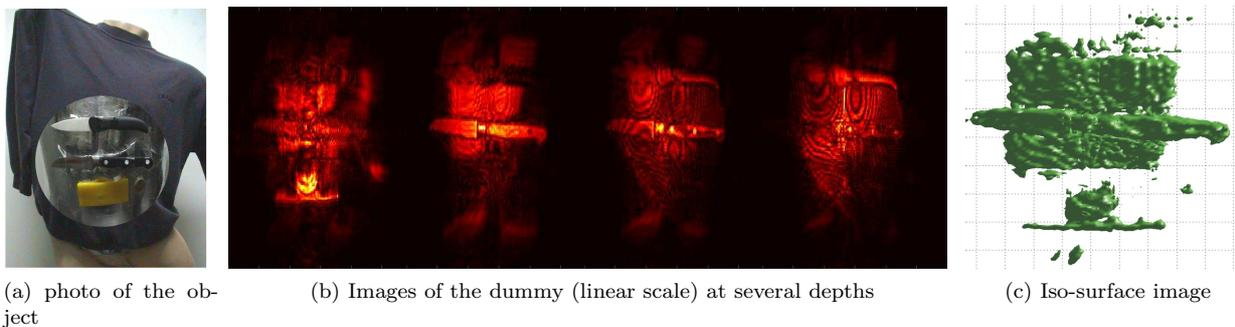
Fig. 3: PVC dummy packed with a metallic knife, ceramic knife and a explosive simulant, everything covered with a pullover
