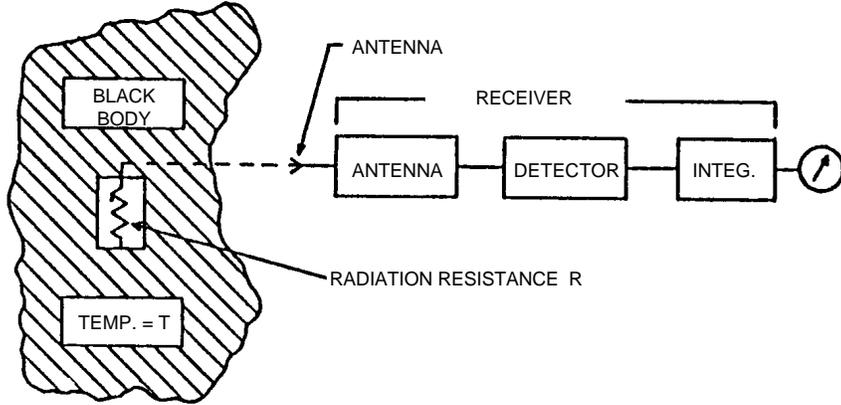
Figure A-2: Simplified block diagram of an antenna and receiver. When the antenna is immersed in a blackbody at temperature T, the receiver input is equivalent to a resistive load R immersed in a thermal bath at temperature T.
