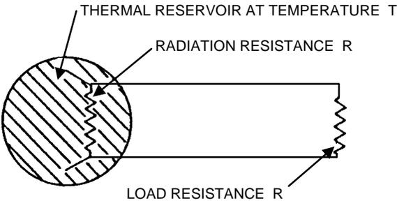
**Figure A-1:** Equivalent circuit of an antenna immersed in an absorbing medium at temperature  $T$ . In equilibrium, the temperature of the load resistance is the same as the temperature of the absorbing medium.
