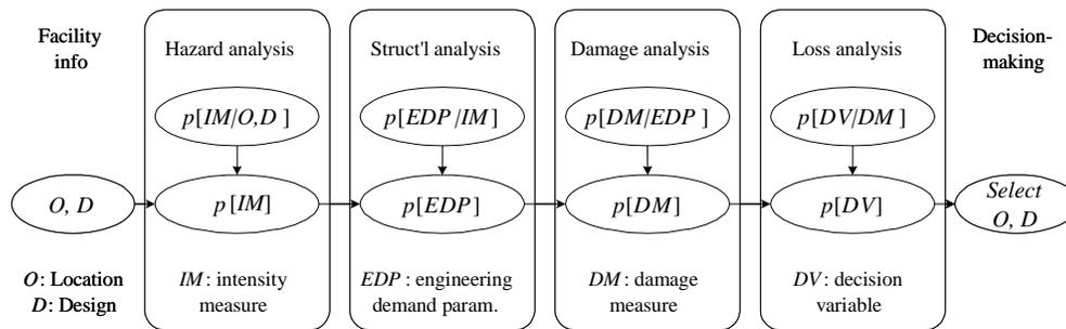
Figure 5. Probabilistic underpinnings of the PEER and ATC-58 performance methodologies (Moehle 2003)
